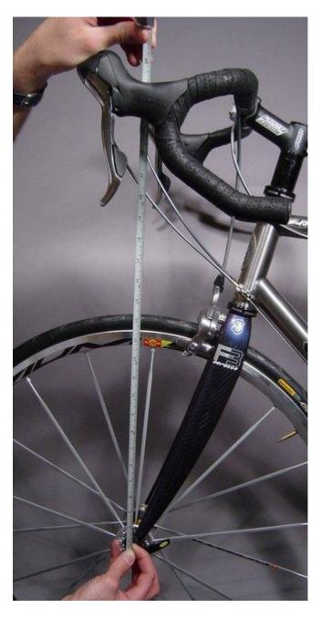
• Faxle to HB c ( Front axle to Handle Bar center ) — As this statement implies, we measure from the front axle to the center of the handle bar @ the stem junction. To ensure an accurate measurement, make the line as direct as possible around cables.
