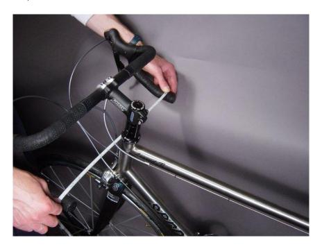
• *HB angle* ( <u>Handle Bar</u> ) – We measure the angle of the handle bar by placing an angle protractor on the bar at the same spot where we take the width reading. (Keep in mind that grip tape variation will affect your measurement!)
