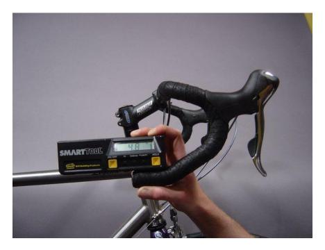
• *Grip height* – This number is determined by measuring from the center of the front axle to the top of the brake/shifter hood, where the hand naturally settles.
