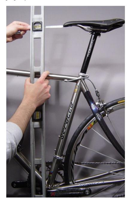
• Saddle HB differential ( <u>Handle Bar</u>) – You'll need your level again for this one! This measurement is taken to determine the how much higher or lower the saddle is in relation to the handle bar. Using the level, place one end on the higher of the two surfaces. While resting on that surface, level it out and measure from the bottom edge to either the top of the saddle or to the handle bar.
